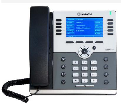
Infinity 5010 - 10 button, innovative Gigabit Color IP Phone, with a 4.3" TFT-LCD - 480x272 pixel display.
